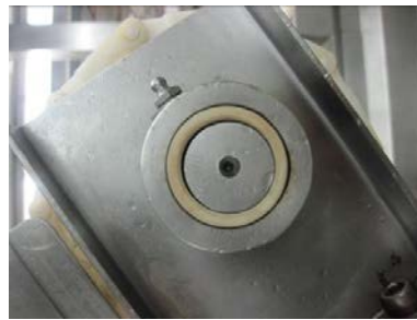
Greaseless Thordon SXL bearing
