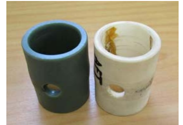
Left existing Nylon bearing, right Thordon SXL bearing
